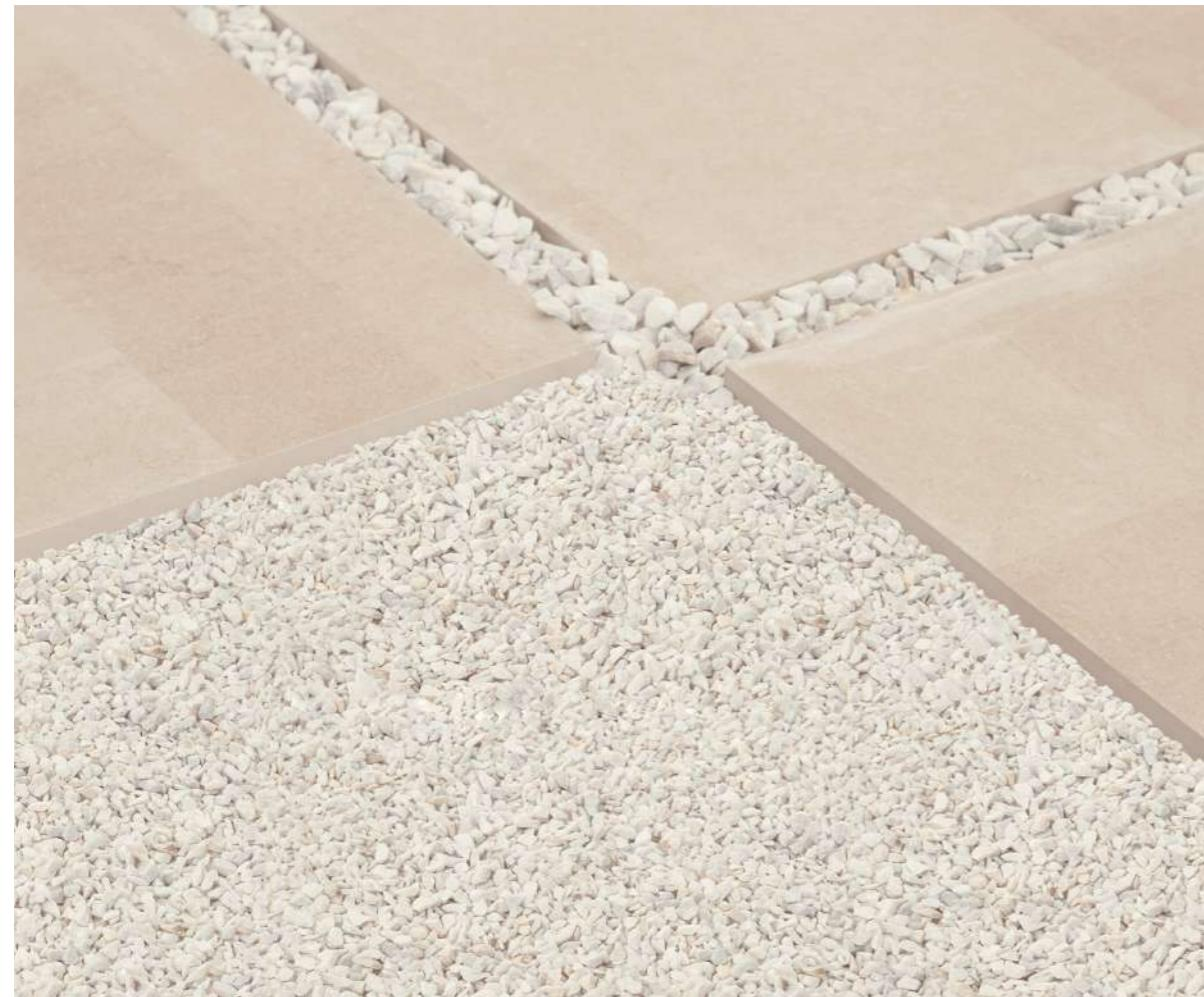
**EN** Perfect for courtyards, patios and places requiring good drainage. Lay the tiles on top of a layer of fine, compacted, level gravel. If you leave tile joints of +/- 5 cm, fill them with more gravel to stop the tiles from moving. If the joints are +/- 5 mm, fill them with sand.
