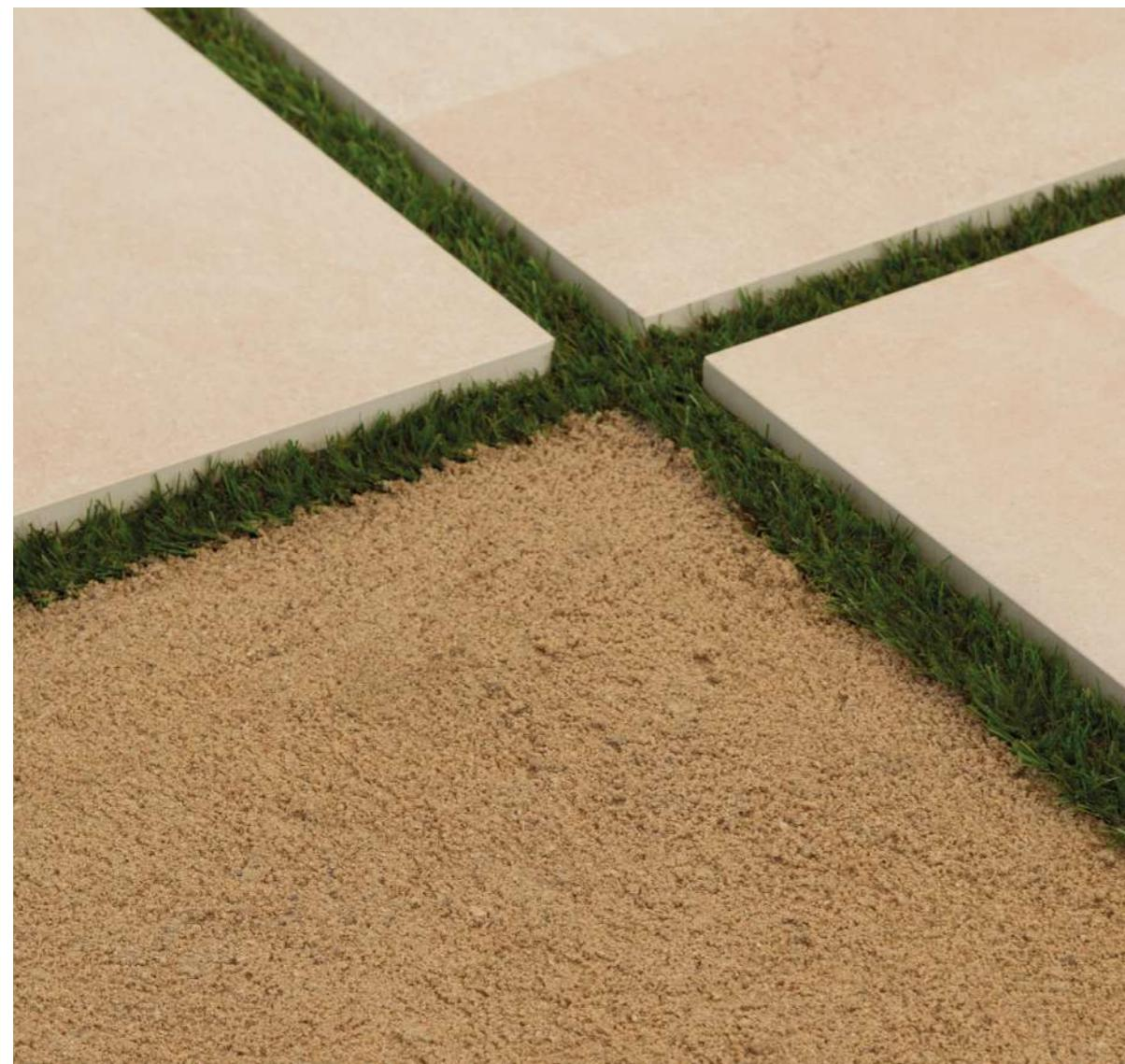
**EN** This is the simplest tile-laying method. Just dig down to a depth of 5 to 10 cm, fill the space with fine gravel or compacted sand, and lay the tiles on top. Tile joints of between 5 and 10 cm can be left so that grass can grow between the tiles.
